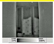
**Above:** Infrared scan of poorly installed, mice ridden, ineffective insulation. **Below:** Cellu-Spray fixing a similar problem.
